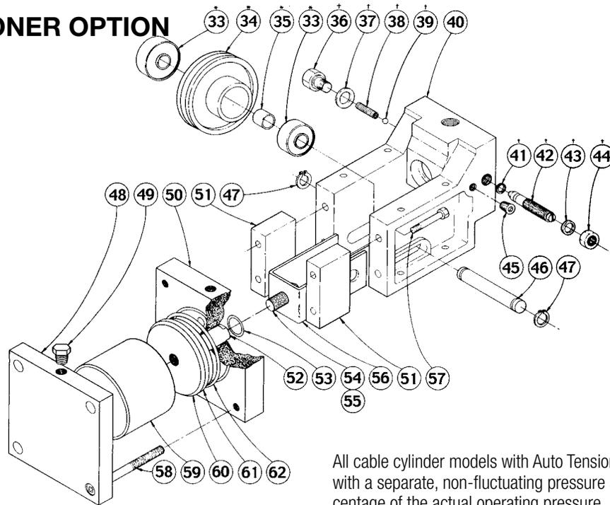
All cable cylinder models with Auto Tensioner units should be plumbed with a separate, non-fluctuating pressure source which is a set percentage of the actual operating pressure.
