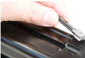
Place switch bracket into one of the four slots that run the length of the extruded tube. Note that there is a cutout on the actuator head (RSA) or tube (GSA) to allow insertion of the bracket. Insert the switch with the word "Tolomatic" facing up and slide it under the bracket. Position the bracket with the switch to the exact location desired, then lock them securely into place by tightening both set screws on the bracket.
