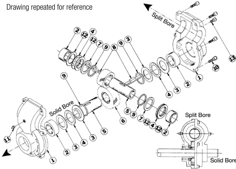
Gear (6) over the Sleeve Bushing (5) positioning it over Key (8). Install Plastic Spacer (9) and a Nylon Ring Spacer (7) on both sides of gear. Lubricate all bearings and the Gear (6) manually (See "Lubrication"). Install a Thrust Washer (12), Thrust Bearing (4), and Thrust Washer (12) on each side of gear. Install a Roller Bearing (2) on each side of Gear (6). Lay the completed assembly into the split bore of the Gear Case Housing (1), making sure the teeth of the gears mesh.
