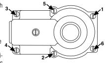
**Lubrication:** All Float-A-Shaft<sup>®</sup> gear boxes have been lubricated at the factory with Mobilith® SHC 460. However, units require more lubrication prior to operation. Periodic re-lubrication is also necessary for optimum performance. When re-lubricating, inject Mobilith® SHC 460 (maximum operating temperature of 300°F or higher and EP rated) into gear case, as required, via the grease zerk provided. *Mobilith® SHC 460 - 14 oz grease cartridge • P/N 0100-1605*
