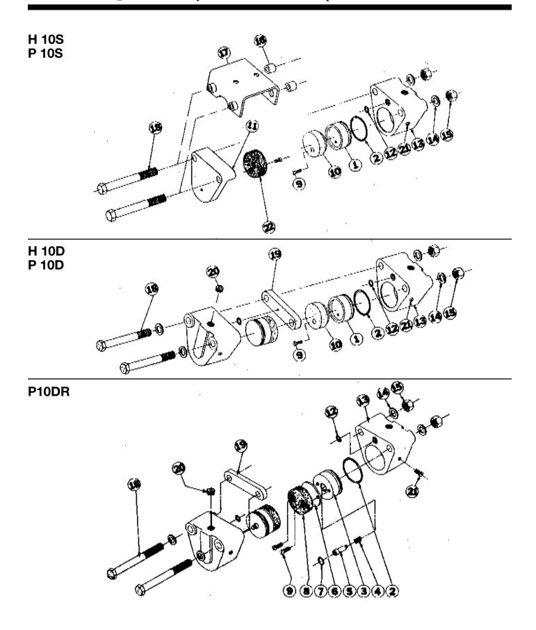
Note: Hydraulic models purchased prior to February 1, 1988, utilitze O-Ring seals on bleeder screws. Hydraulic models purchased after that date use Nylon sealing washers.
