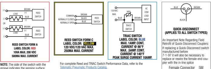
NOTE: The side of the switch with the groove indicates the sensing surface. This must face toward the magnet.
