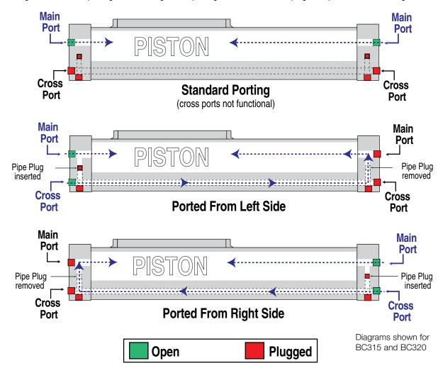
Note: Standard porting may be field converted to ported from left or ported from right. For complete instructions refer to parts sheet.
