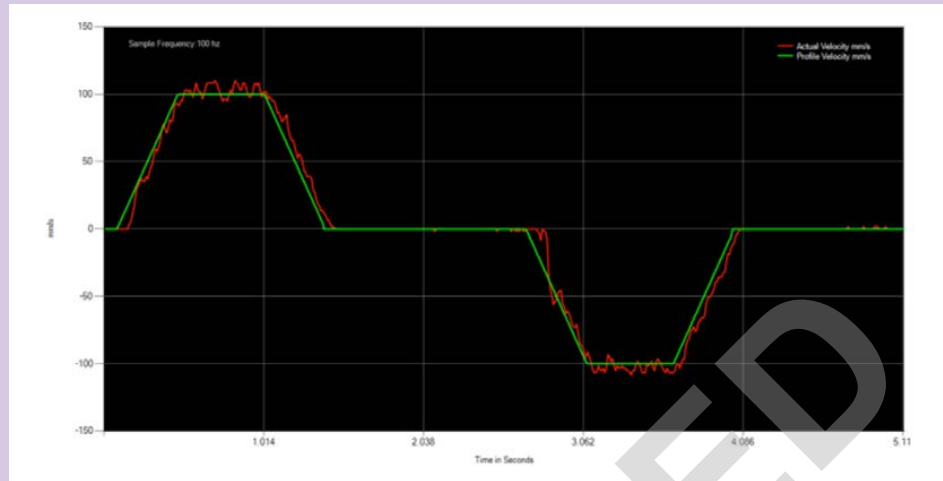
Figure 16-16: Velocity Integral Gain - Too High: Oscillations
