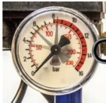
Air pressure increased to compensate for low weld force
