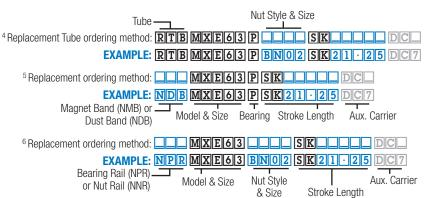
Auxiliary Carrier Option Note: If replacing a Tube (1.), Dust Band (2.), Magnet Band Kit (3.), Bearing Rail (4.), Nut Rail Kit (5.), or Lead Screw (28.) on an actuator that has an Auxiliary Carrier, be sure to add "DC \_ \_ \_" to the end of the configuration string when ordering. "DC" indicates the need for additional length and "\_ \_ \_" indicates the measurement of space between carriers (in inches [SK] or millimeters [SM] as indicated earlier in the configuration string).
