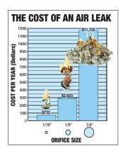
Cumulative air leak in a facility from all sources. Costs calculated using the industrial electricity rate of \$0.07 per kWh\*, assuming a consistent operation and an efficient compressor.
