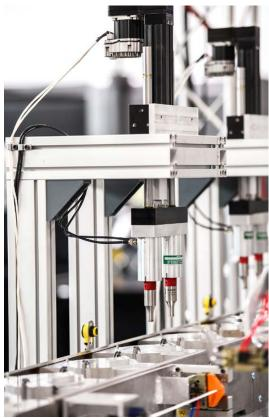
Tolomatic GSA actuators (positioned above masks) provide motion function to apply elastic ear straps. Photo: Tolomatic, Inc.
