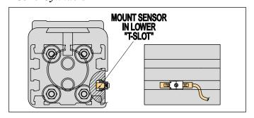
Two "T" slots are located on each side of the cylinder extrusion. Installing the sensor in the lower "T" slot, will allow the sensor to be positioned appropriately to accommodate "full end of stroke" sensing.
