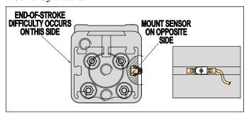
The piston has been fitted with two magnets, each on opposite sides of the piston. Install the sensor in the cylinder "T" slot on the opposing side of the cylinder. The magnet on that side will activate the newly intalled sensor and allow "full end-of-stroke" sensing capability.
