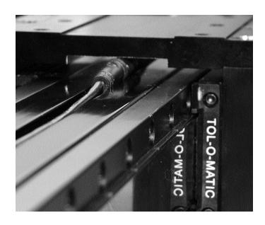
When using the Dual 180 option on BC3, B3S, B3B. and B3W actuators, there may be a space constraint encountered when installing and subsequently routing the wires for switches under the Dual 180 connector bracket.
