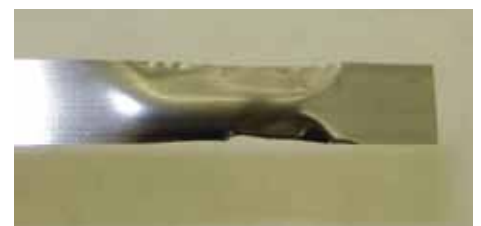
The actuator's sealing band experienced cupping damage caused from inertia spikes.
