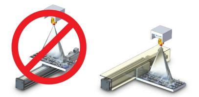
Figure 3: The above application depicts a spray head with direct spray contact to the rodless actuator. The illustration on the left shows a rodless actuator with no shielding. The illustration on the right shows the proper shielding a rodless actuator would require for direct spray applications.
