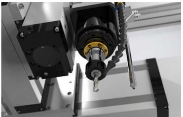
The RhinoFab 9-axis fabrication machine moves nine different axis points: three each on the top, bottom and front – each accommodating up to three different tool sets – to fabricate the storefront and curtainwall material. The machine can fabricate from the top and bottom at the same time.
