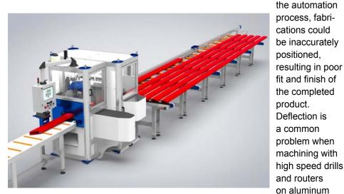
The 9-axis RhinoFab glazing machine, which pre-drills and cuts lineal materials to spec, is designed to deliver the required force and pressure to drill perfectly placed holes and route intricate patterns.
