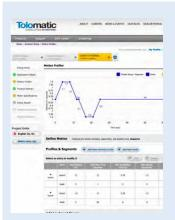
Sizing software works through all the complex equations to evaluate the static and dynamic influences on an actuator in an application.
