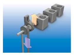
This illustration shows the mounting configuration of the existing timing belt mechanism, pillow block, and their relation to the first Slide-Rite gearbox on the shaft line.
