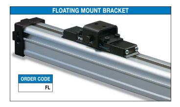
For applications where a BC4 band cylinder is moving a load that is externally guided and supported. An externally guided load, not parallel to the BC4 band cylinder may result in cylinder binding. The floating mount bracket compensates for nonparallelism between the cylinder and the external guide.
