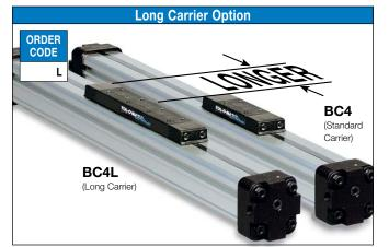
Long carrier option greatly increases the "My" and "Mz" moment load capacity. This broadens the application range for these models. Other benefits include larger mounting surface and virtual elimination of chatter for vertical cantilever loads.
