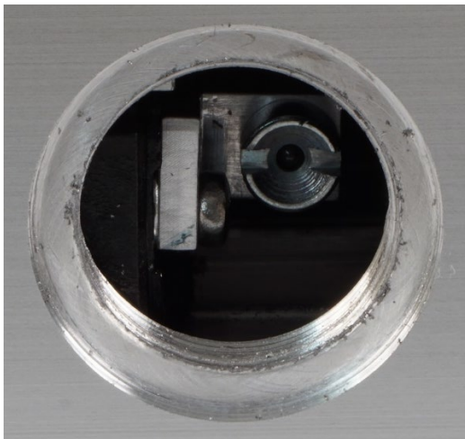
Figure 6.3: Position the carrier to permit lubrication of each of the 4 linear bearings
