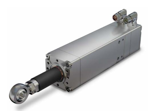
The IMX Servo Linear Actuator delivers up to 26 kN (5,850 lbf) of force in a patented compact design with a built in high torque motor driving precision screw technology,
